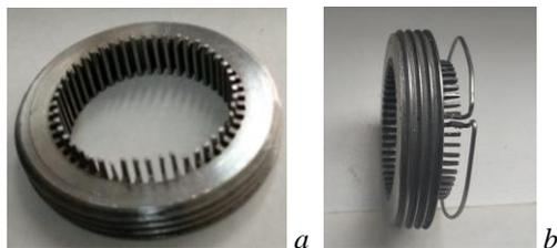
Fig. 5. The EDS of RM-48 with different output elements ('antennas'): rods (a) and a wire ring (b)
