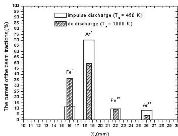
Fig. 4. Comparison of the intensities of different fractions of the ion beams
