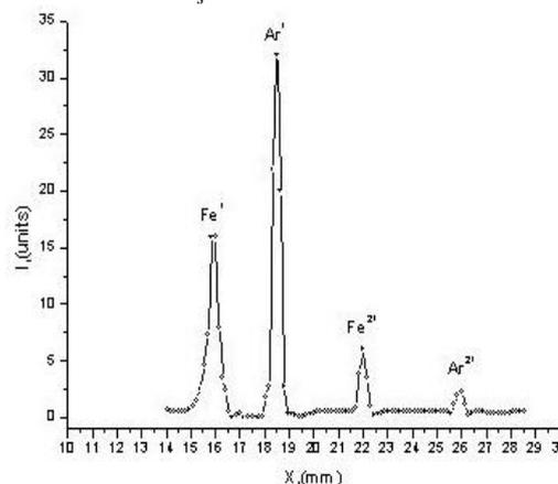
Fig. 3. Mass and charge spectrum of the ion beam. Temperature Penning's anode is 1800 K
