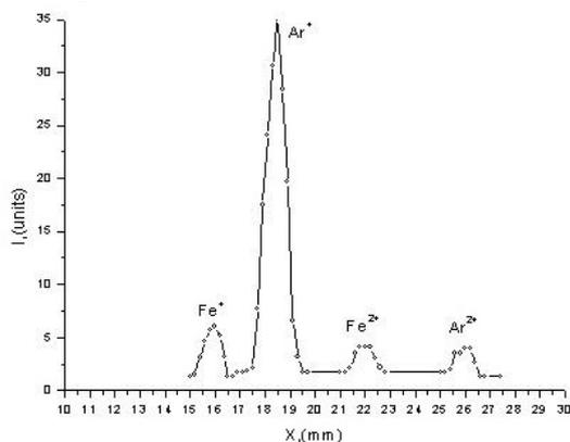
Fig. 2. Mass and charge spectrum of the ion beam. Temperature Penning's anode is 450 K
