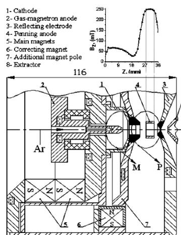
Fig. 1. Design of the sputtering type metal ion source and distribution of magnetic field  $B_z$
