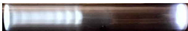
Fig. 12. Photograph of dc discharge for a current of 3 mA and a distance between the electrodes L = 350 mm
