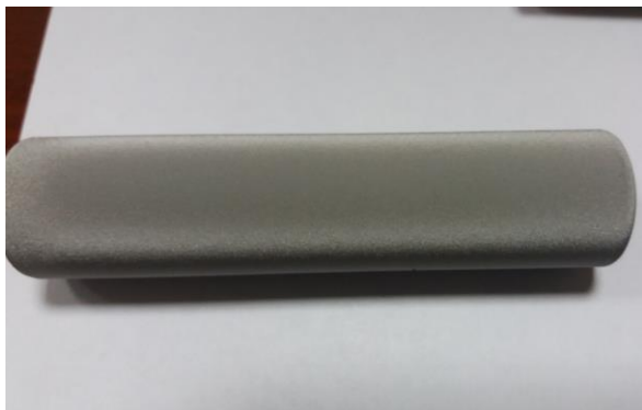
Fig. 1. A sample of tungsten-coated cathode on the graphite substrate
