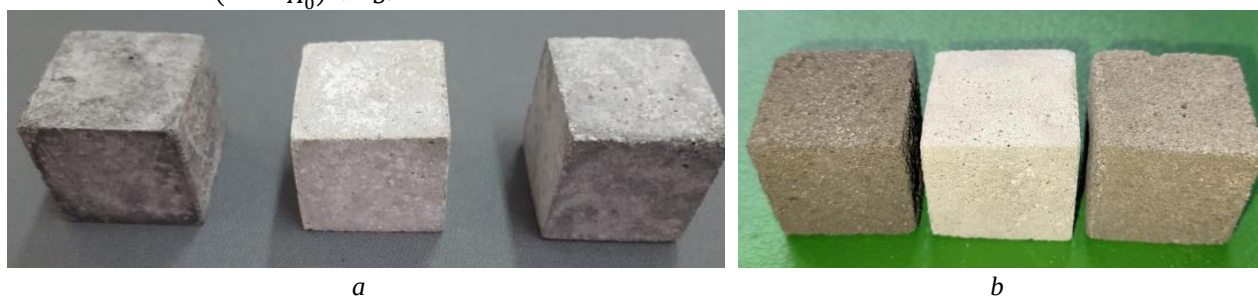
Fig. 1. Samples MKPC-F, MKPC-S, and MKPC-FS (from left to right): a – before, b – after leaching for 1 year
