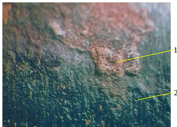
Fig. 6. A layer of deposits on the HET in the lower part of the SG (see Fig. 3,a, position N 1)
