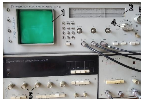
Fig. 4. Appearance of the panoramic VSWR meter R2-53: 1 – ETL screen; 2 – measurement scale; 3 – handle for moving the reference line; 4 – switch for measurement limits; 5 – knob for setting the frequency values of the reference marks
