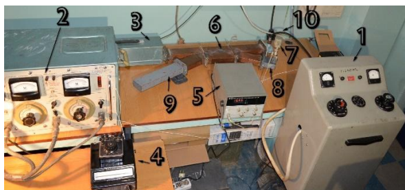
Fig. 6. Stand for measuring microwave power: 1 – generator “Luch-58”; 2 – measuring block of the M3-13/1 wattmeter; 3 – calorimetric load of the M3-13/1 wattmeter; 4 – M95 microammeter, 5 – M3-54 wattmeter; 6 – microwave power coupler from the “VOLNA” installation; 7 – calorimetric converter of the M3-54 wattmeter; 8 – coaxial-waveguide transition (CWT) of the incident power arm; 9 – matched load on the VSWR; 10 – input of microwave power from the “Luch-58” generator
