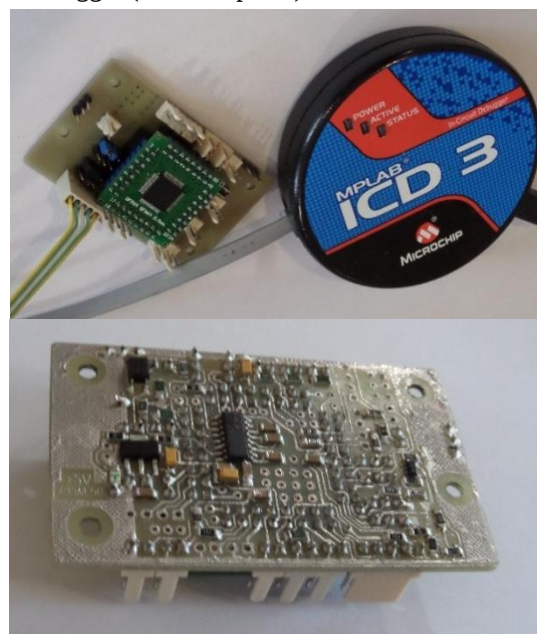
Fig. 5. Programmer (top) and printed circuit board with microcontroller (bottom)
