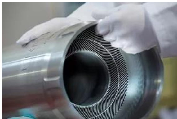
Fig. 5. Reactor fuel element [26]
