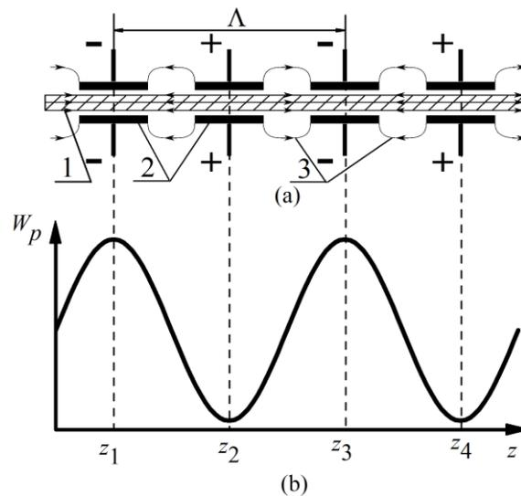
Fig. 2. Scheme of the amplification section for the SCWs: 1 – relativistic electron beam; 2 – electrostatic undulator's electrodes; 3 – electric lines of force of the external periodic reversible pump electric field (a); dependence of the potential energy of beam's electrons  $W_p$  in the external pump electric field  $E_{20}$  on the longitudinal coordinate  $z$  (b)
