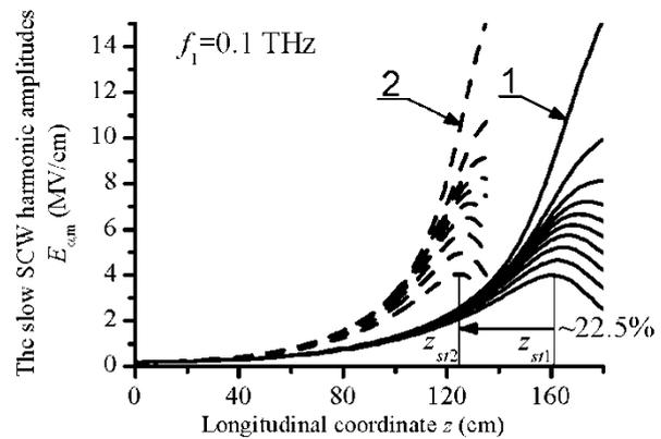
Fig. 4. Dependences of the harmonic amplitudes of the slow SCW's electric field strength on the coordinate  $z$ .
