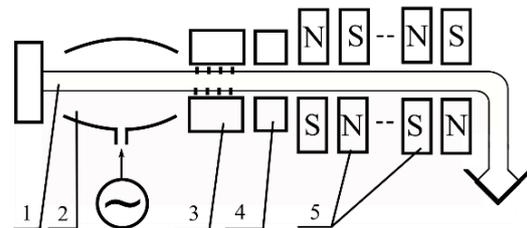
Fig. 1. Scheme of a parametric superheterodyne FEL with a longitudinal electrostatic undulator: 1 – electron beam; 2 – non-resonant modulator; 3 – amplification section of multi-harmonic SCWs; 4 – electron beam acceleration section; 5 – H-ubitron undulator
