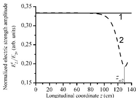
Fig. 3. Dependence of the first harmonic amplitude of the generated pump electric field strength, normalized to the external pump electric field strength, on the longitudinal coordinate  $z$ . Line 1 is built based on the linear approximation equation (14), and line 2 is made based on the nonlinear equation (14)
