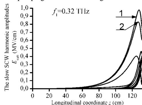
Fig. 5. Dependence of the harmonic amplitudes of the slow SCW's electric field strength on the coordinate  $z$ .
