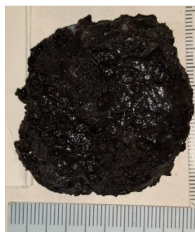
Fig. 3. Original appearance of sample of S080403. Size of grains of component: Al – 10...20 \mu\text{m} , W – 50...60 \mu\text{m}
