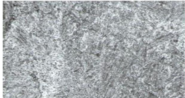
Fig. 7. The structure of the area of incomplete recrystallization of the HAZ of the welded joint of the experimental sample of the rotor,  $\times 400$
