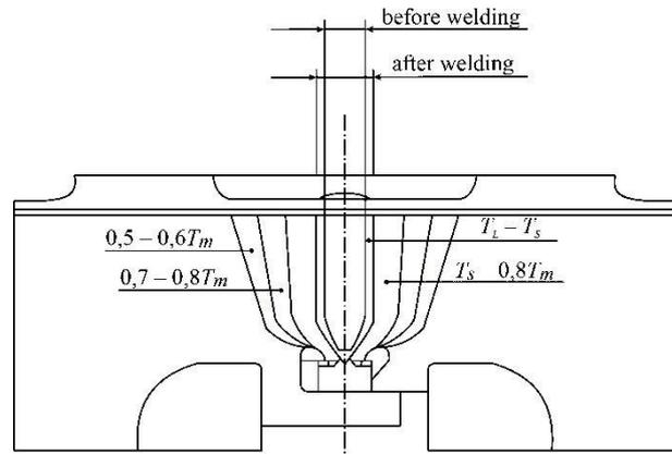
Fig. 3. Fragment of the calculated temperature fields in the pilot sample of the welded connection of the rotor
