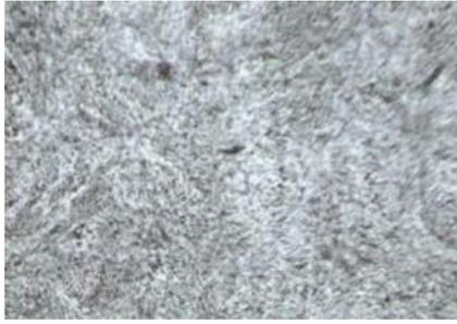
Fig. 2. Initial steel structure 25X2HMΦA, ×360
