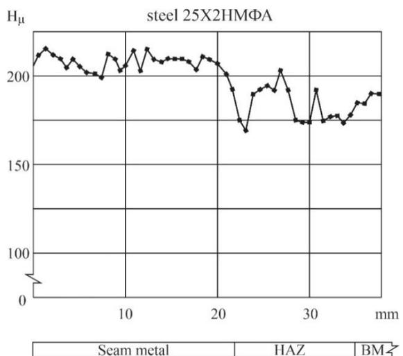
Fig. 8. Distribution of microhardness along the cross-section of the pilot sample of the welded rotor joint
