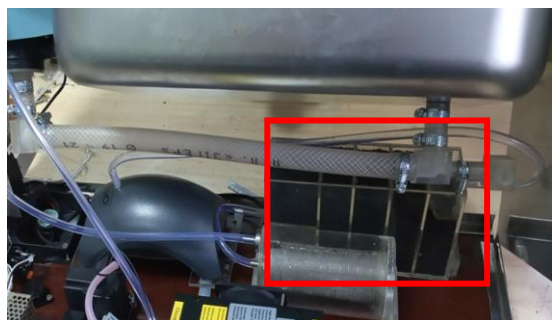
Fig. 1. Ozone destructor inside the sterilizer
