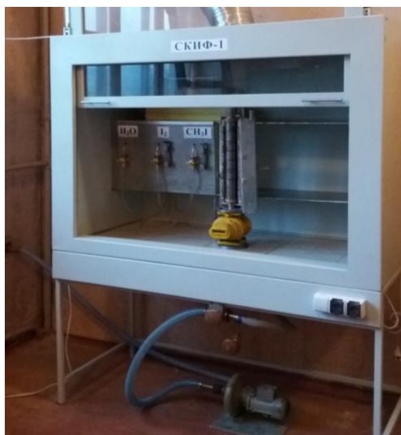
Fig. 3. Pumping module of the SKIF stand
