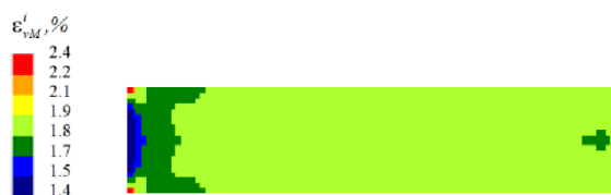
Fig. 3. Distribution of the of irreversible von Mises strains along the plate at t=324,928 h
