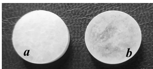
Fig. 2. The photograph of p -terphenyl polycrystals with a diameter of D = 20 mm and a thickness of h = 5 mm obtained by hot pressing of: a – crystalline grains; b – a fragment of a quasi-crystalline ingot
