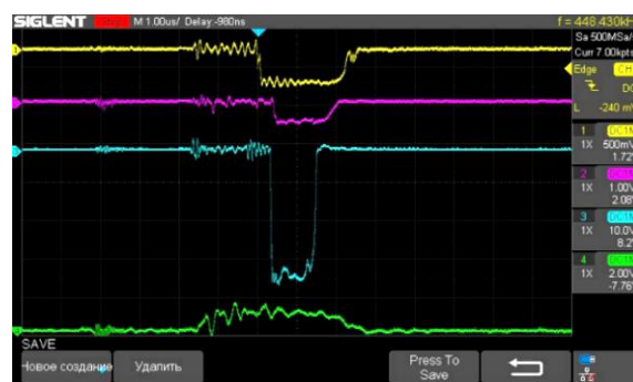
Fig. 1. Accelerator control circuit (a) with output oscillograms (b). The yellow beam is a pulse from the “Rubin” generator detector. The violet beam is a pulse at the klystron cathode. The blue beam is a pulse from the Faraday cup. The Green – impulse from the current sensor at the output of the electron gun
