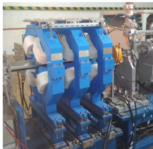
Fig. 18. Quadrupole magnet of the accelerator transportation channel
