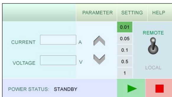
Fig. 35. Power supply local control panel
