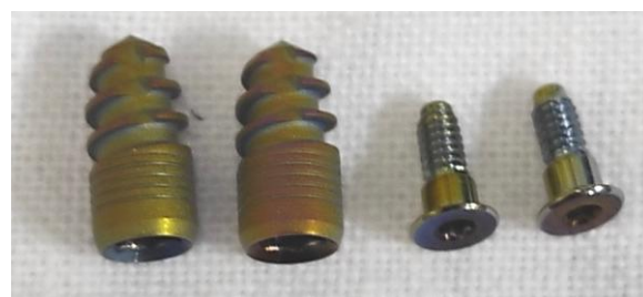
Fig. 3. Image of ZrTa/ZrTaO 2 coatings on Ti dental implants
