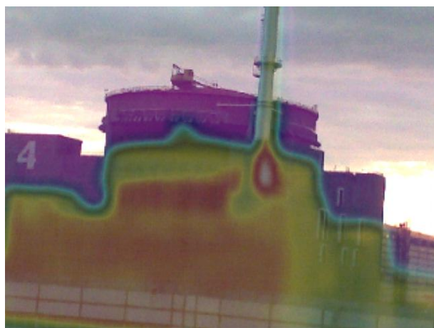
Fig. 1. Panoramic thermogram of the nuclear power unit
