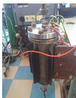
Fig. 2. General view of the E-2 chamber (a); electrolysis module (b): 1 – anode; 2 – cathode; 3 – fluoroplastic insulator; 4 – electrolyte; 5 – flange fitting
