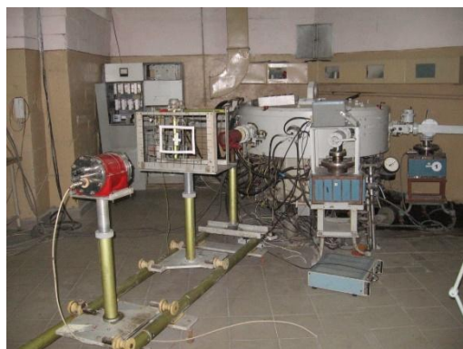
Fig. 1. The M-30 microtron as a metrological test bench for radiation experiments
