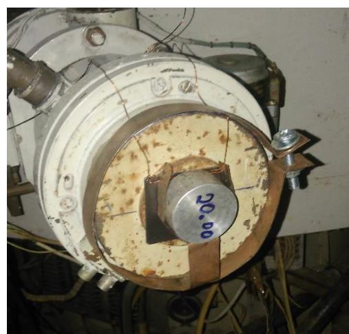
Fig. 2. Scheme of stimulation of the ^{19}\text{F}(\gamma, n)^{18}\text{F} reaction on the M-30 microtron – a: 1 – block of electron extraction; 2 – window of the output node (ellipse 22x6 mm, thickness – 50 \mu\text{m} ); 3 – Ta-converter (52x45x1 mm); 4 – aluminum filter (diameter – 30 mm, thickness – 20 mm); 5 – hermetically packed Teflon samples and b – photo of the output node
