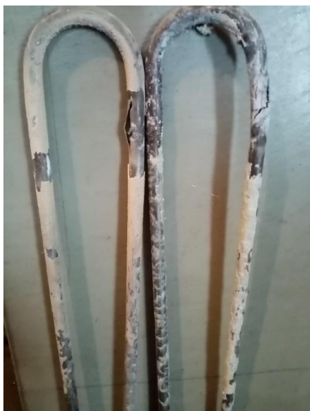
Fig. 3. Appearance of heaters removed from the accelerator
