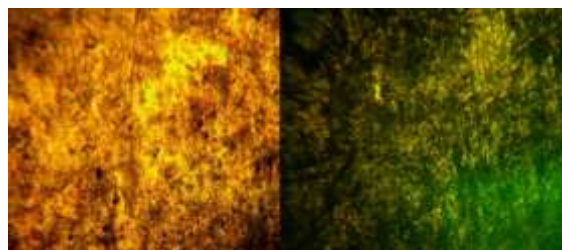
Fig. 8. Steel 12X18N9T EPP processed after the cathode process in which the sample melted anodic process (magnification \times 160 )
