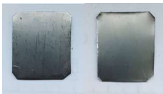
Fig. 2. The 12X18H9T stainless steel images before (left) and after EPB (right)
