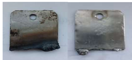
Fig. 9. Images of steel 12X18N9T before (left) and after (right) EPP anodic treatment
