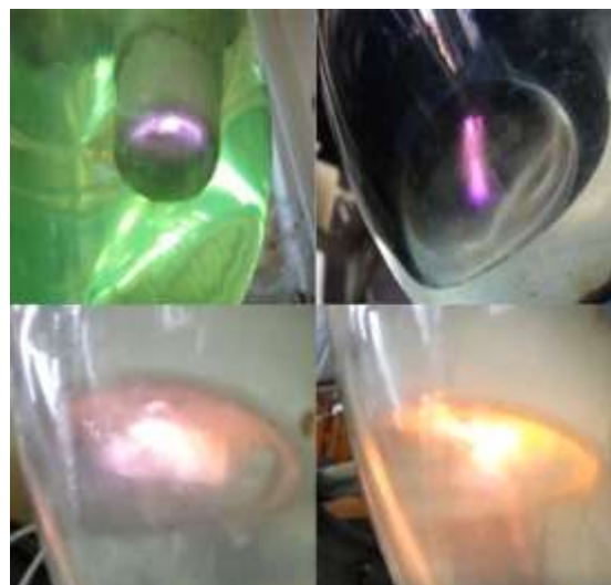
Fig. 3. Photos of high-voltage pulsed discharges in gas bubbles during water treatment
