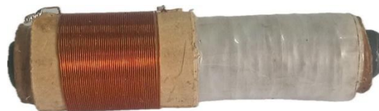
Fig. 3. The main view of the transformer
