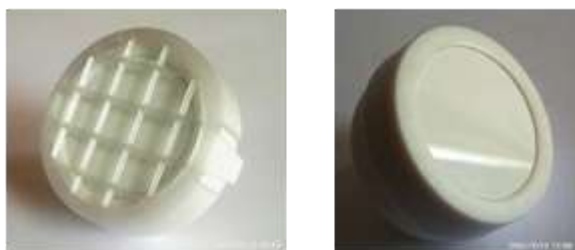
Fig. 2. Reactor module with a nozzle manufactured by using 3D printer
