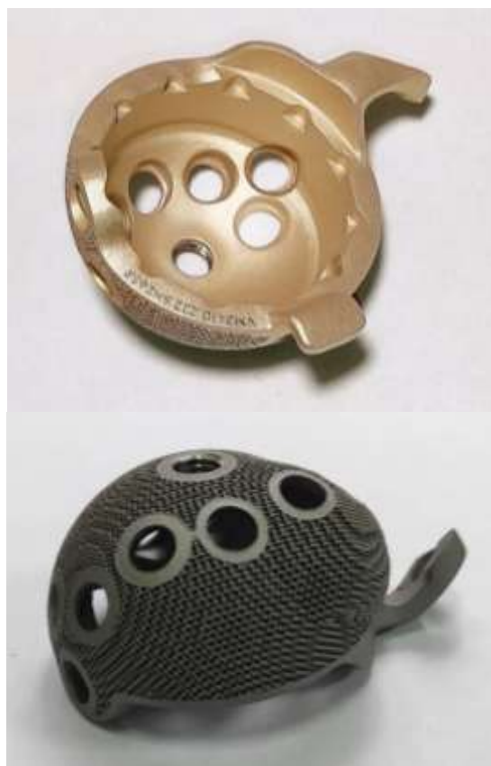
Fig. 2. Titanium hip implants (top – coated, bottom – uncoated)
