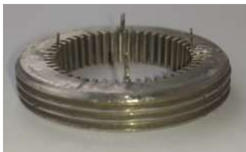
Fig. 3. Version of power emitting structure with four rod “antennas”
