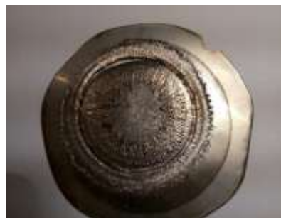
Fig. 4. Tubular REP imprint on a stainless steel converter after 5 pulses
