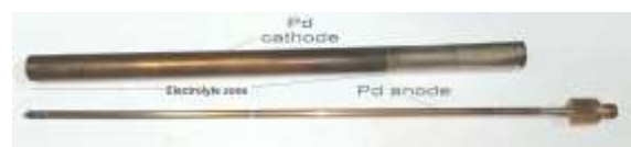
Fig. 2. Cathode and anode after one-hour exposure to electrolysis current
