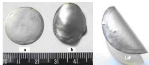
Fig. 11. The sample shape change after hydrogen saturation [8]: a – before saturation; b – after 62 h saturation; c – after 150 h saturation
