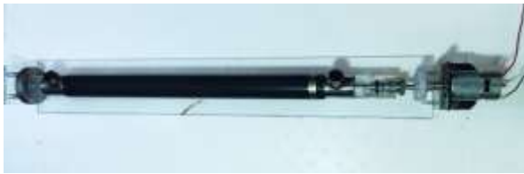
Fig. 6. Photo of a plasma-chemical reactor with a rotating cathode driven by an electric motor
