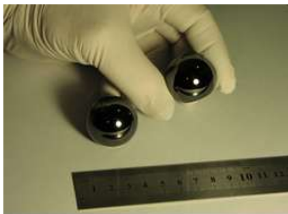
Fig. 5. Hemispherical components of friction units of artificial joints with wear-resistant DLC coating
