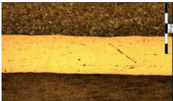
Fig. 4b. Batch method of producing bimetal, copper layer thickness 400 \mu\text{m}
