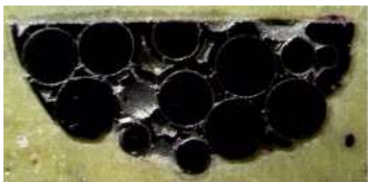
Fig. 9. Segment of a frame made of steel spheres impregnated with pyrolytic chromium by vapor deposition. The diameter of the spheres is 1 mm. The density of filling the volume with spheres before the process was 0.64
