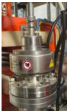
Fig. 14. Pressure probe with cold cathode (IKR - 050)
