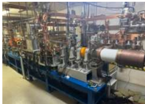
Fig. 1. The first section of the electron accelerator (right view)
