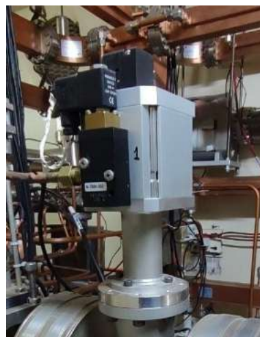
Fig. 16. Fast gate valve DN 16–40
