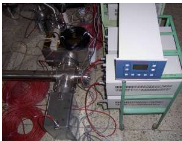
Fig. 12. Power supply source and control unit SP-D/T with ion pump
