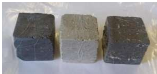
Fig. 1. MKPC-FA, MKPC-BFS and MKPC-FA-BFS specimens (from left to right) after leaching in an alkaline solution for 90 days
