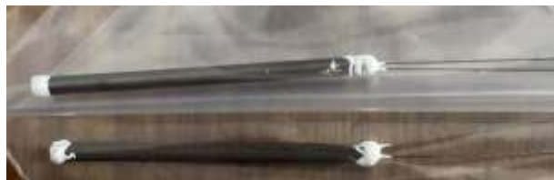
Fig. 3. Detector samples with a diameter of 2.5 mm for testing
