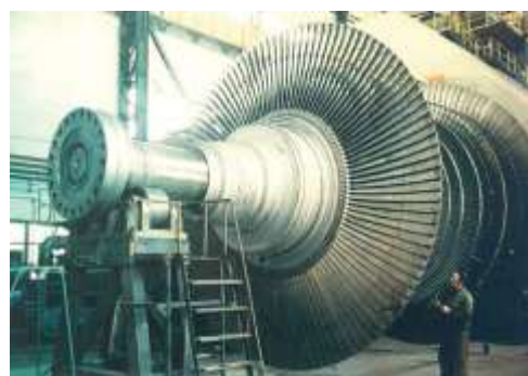
Fig. 2. Low-pressure turbine rotor K-1100-60/1500-2M
