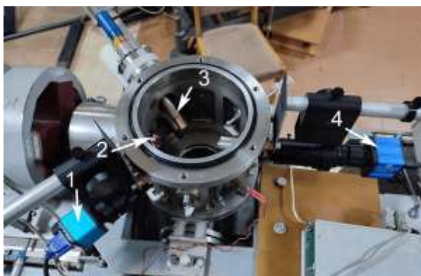
Fig. 2. Exterior view of the target chamber with the installed equipment. 1 – front video camera; 2 – LED backlight; 3 – XRD detector; 4 – rear video camera
