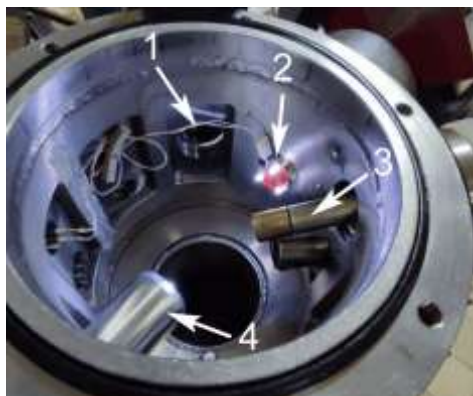
Fig. 3. Internal view of the camera with the installed equipment. 1 – location of the front video camera for positioning monitoring; 2 – LED backlight; 3 – CBR detector; 4 – location of the rear video camera for focusing
