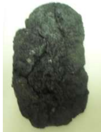
Fig. 4. Original appearance of sample of CFe050901. Size of grains of component: Al – 10...20 \mu\text{m} ; Fe – 230...280 \mu\text{m}
