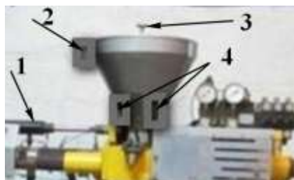
Fig. 1. Photograph of feedstock feed system and bunker with improvements: 1 – feedstock feed motor and system of rotation; 2 – mixing system motor; 3 – IR camera for control of heating; 4 – heaters
