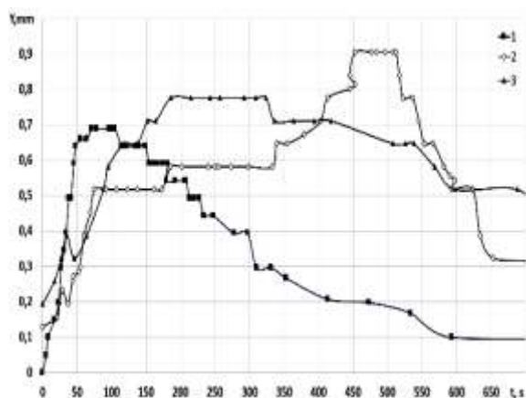
Fig. 3. Time dependences of cantilever shape change: 1 – for pure palladium; 2 – for \alpha\text{-PdH}_{0.0077} alloy; 3 – for \alpha\text{-PdH}_{0.0177} alloy at a hydrogen injection rate of 4.8 \cdot 10^{-5} MPa/s
