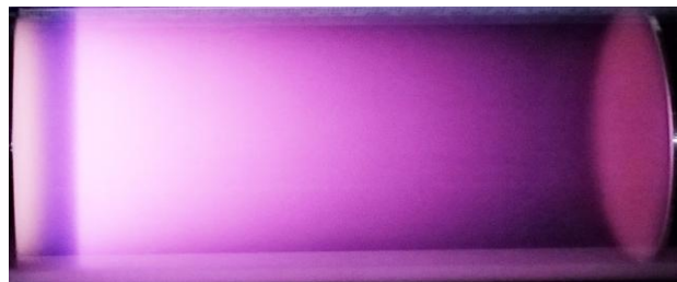
Fig. 5. Photograph of the discharge at a \text{CF}_4 pressure of 9.3 Pa, current of 5 mA, and distance L = 140 mm. The cathode is on the left, the anode on the right. An anode glow appears near the anode surface
