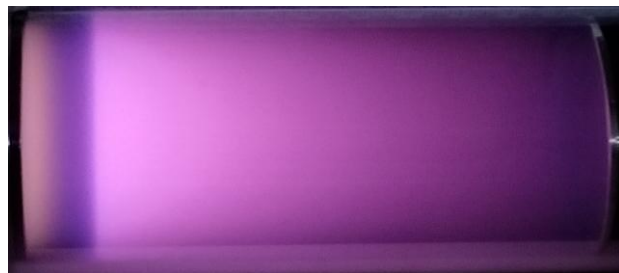
Fig. 4. Photograph of the discharge at a \text{CF}_4 pressure of 9.3 Pa, current of 5 mA, and distance L = 110 mm. The cathode is on the left, the anode on the right
