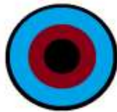
Fig. 1. Geometry of coaxial ferrite line. Black shows inner and outer conductors, brown shows ferrite layer, blue shows dielectric layer
