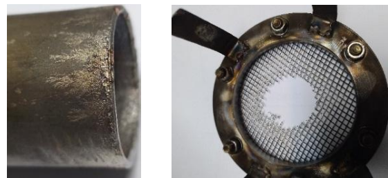
Fig. 7. Photo of the processes at the cathode end (left) and photo of the interaction of the beam with the anode grid
