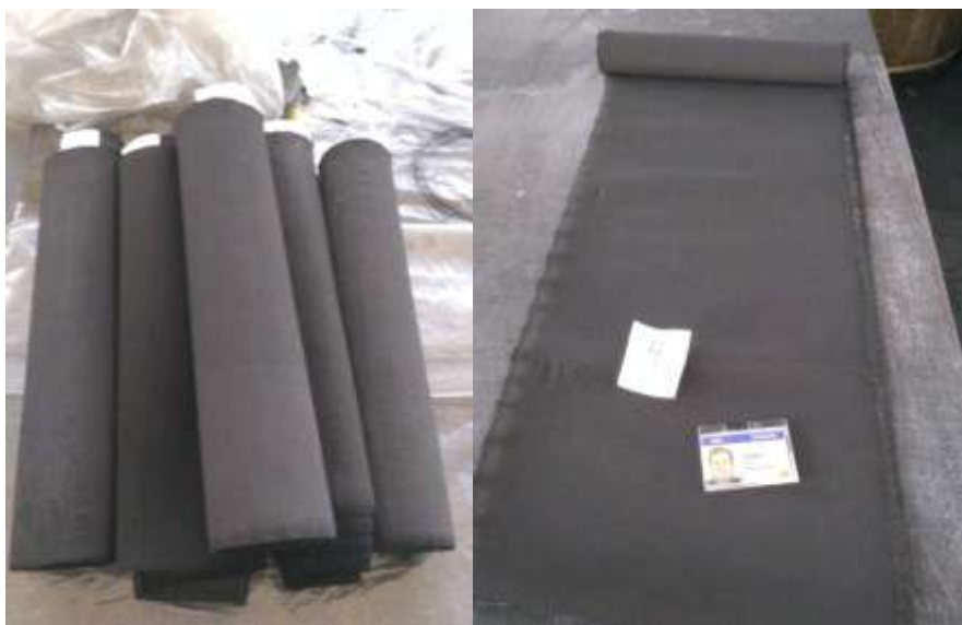
Fig. 5. Appearance of the activated carbon fabric obtained from the precursor “tarpaulin harsh cotton/Jute 470”
