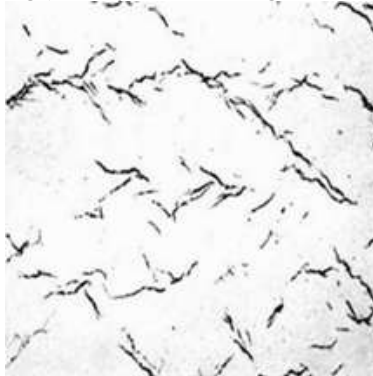
d – furnace cooling (more noticeable stack hydrides, with significant reorientation)
