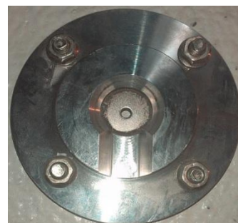
Fig. 7. Accelerator tunnel wall target-reflector holder of the NSC KIPT SCA "Neutron Source"
