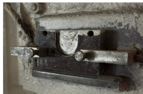
Fig. 6. Target-reflector holder at the wall of the SCA facility at the experimental hall (Base 1, Base 2, Base 3)
