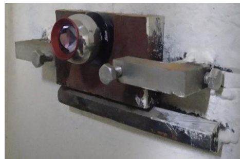
Fig. 5. Target-reflector holder at the beginning of the accelerator tunnel (Egun)
