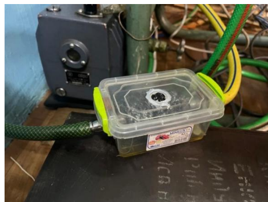
Fig. 3. Additional reservoir installed at the outlet of the forevacuum pump
